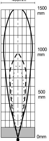
DUPR-A sensors are shown (small, medium and large cone). Furthermore, the size of the detection beam is influenced bν temperature and humidity. The colder and dryer the air, the larger is the beam.
